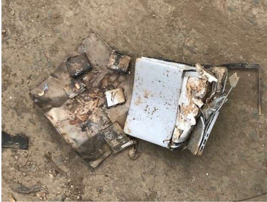
This photo shows the remains of a laptop that was dropped into a curbside recycling container. During the sorting process at the recycling facility, the Lithium Ion battery in it exploded and caught fire.
