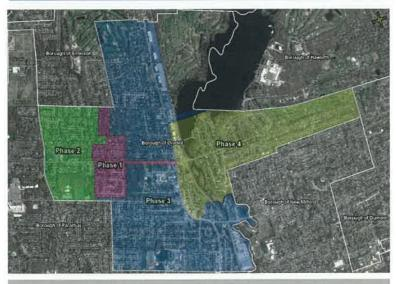
Services included the design for a multi-phased sewer improvement project, including televised inspection and analysis of approximately 196,500 linear feet of pipe. Boswell prepared the contract documents for the replacement of 5,400 linear feet of pipe and lining of approximately 22,000 linear feet of existing sewer. Ground penetrating radar (GPR) was utilized to determine the depth and location of utilities during design to minimize utility conflicts during construction.
